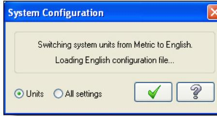
Mastercam switches the configuration file to `mcamx.config <English>`, and the part opens with English units.
