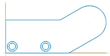
Two of the circles you completed will be used as drill holes and the other two will be used in the next lesson to create the inner shape of the part.
